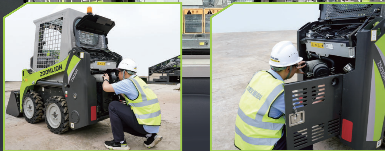
▪ Large upper cover tipping angle for easy maintenance
